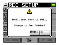
During recording, if you press the REC key to try to start the next take, the next take can be recorded 4 seconds after starting recording when in poly mode or mono subfolder mode. In folder mode, however, some cases will take more than 4 seconds.
