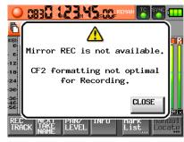
■ During mirror recording, if one of the CF cards runs out of remaining space or has an error, recording to that CF card will stop. Recording of the current take to the other CF card will stop, but recording of a new take as a new file will start immediately.
