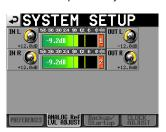
Make fine adjustments to the analog input levels with the INx knobs and make fine adjustments to the analog output levels with the  $\overline{0}UTx$  knobs ("x" is L or R).
