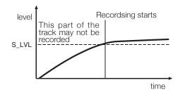
Also remember that when recording from an analog source, the threshold should be set so that it is higher than the "noise floor". If the "noise floor" is higher than the threshold, a false start will occur:
