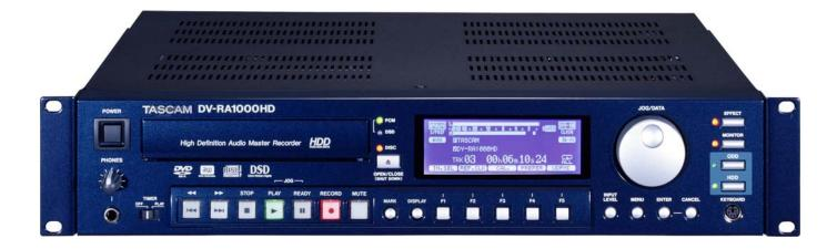
The DV-RA1000HD, 2U rack-mountable, high definition Audio Master Recorder equipped with an internal 60GB hard disk and a optical drive, which records to CD-R/RW and DVD+RW discs, and archives to DVD-R, DVD-RW, DVD+R, and DVD+RW discs. The unit records high quality stereo up to 192kHz/24bit or DSD format to standard CD-DA, Broadcast Wave, and DSDIFF formats. Multi-band compression and 3-band EQ are included; both assignable to record or playback.
