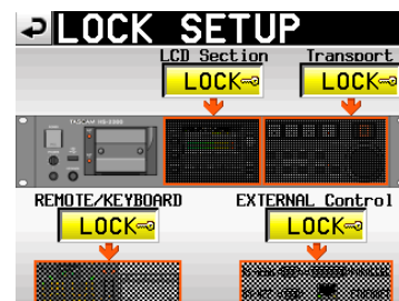
LOCK SETUP screen with all sections locked
