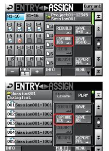
2. Touch the CAPTURE BC\$ button, which has been added to the pull-up menu, to open the following pop-up window message.
