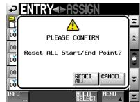
6. Touch the RESET ALL button in the pop-up window to reset the entry's starting and ending times to the beginning and end of the file.
