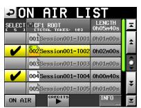
3. The on air list screen shows the audio files that match the set sampling frequency in the root directory of the CF card in file name order.
