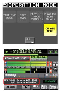
2. In on air mode, the Home Screen shows the names of the next two upcoming takes in the information field. Touch the information field or the take name button to open a pull-down menu, and touch the ON AIR LIST button to open the ON AIR LIST screen.
