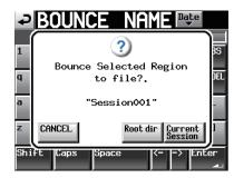
Touch the  ${\tt Root}\,\dim\,{\tt button}$  to save to the root directory of the current CF card.
