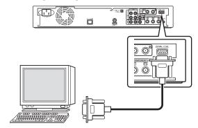
External operation is enabled by connecting a RS-232C cable to a PC or similar device.
