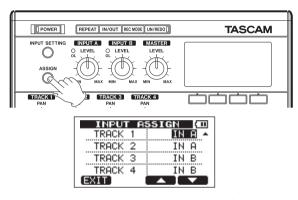
As shown above, the input channel that is the recording source for each track (1-4) is shown. In the initial setting, INPUT A is assigned as the recording source for tracks 1 and 3, and INPUT B is assigned as the recording source for tracks 2 and 4.
