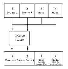
Source tracks are erased when they are bounce destinations. (In the illustration above the drum parts are overwritten by the stereo mix). However, you can use the unit's (undo) function to return to the previous state if you make a mistake (see "Undoing the last operation (single undo)" on page 66).
