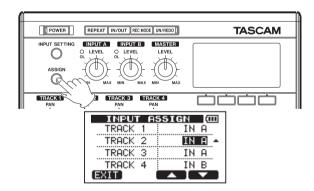
2 Press the F4 (♥) key to select TRACK 3 to change its current input channel from the default of IN A.
