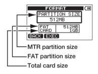
The following table shows the FAT and MTR partition sizes for different SD card capacities. The FAT partition size is set automatically according to card capacity. The size of the MTR partition on cards 4 GB or smaller is also fixed, but cards that are 8 GB or larger have multiple MTR partitions and their sizes can be chosen. However, the last MTR partition is set to fill the remaining space on the card automatically, so its size cannot be chosen.
