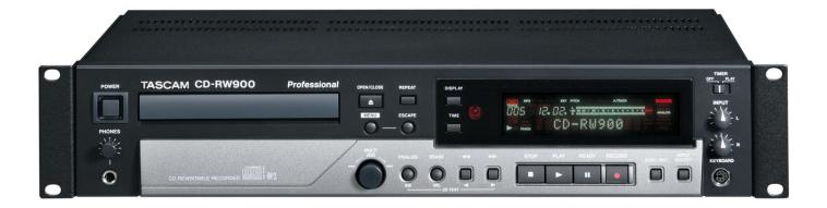
The TASCAM CD-RW900 is a 2U rack-mountable CD Recorder equipped with standard features such as MP3 audio playback, Pitch Control (16 %+/-), and CD Text. The CD recorder provides Key Control (changes the pitch without changing the speed), front PS/2 keyboard input, "Power-on-Play", dedicated analog input level controls, and digital input level control (via multi-jog wheel).
