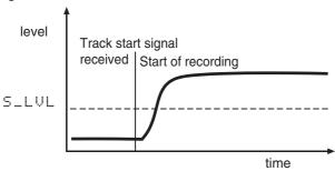
• when recording digitally from a CD or MD deck, a digital track start signal is received, and the signal level subsequently rises above the trigger level:
