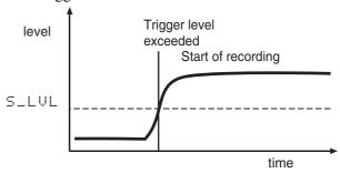
In this last case, if the signal level is already higher than the trigger level, recording starts immediately.
