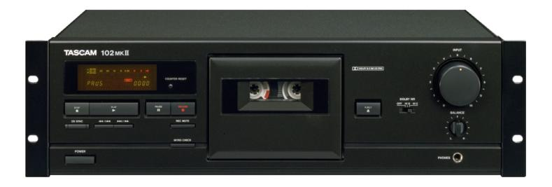
The TASCAM 102mkII is a 3U rack-mountable single well cassette deck utilizing a two-head mechanism for playback and recording. Rear panel inputs and outputs are unbalanced RCA with an input-level control wheel and balance control knob on the front. The cassette offers a single headphone output and Dolby B and C noise reduction with HX Pro Headroom Extension.
