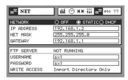
You can see that each screen allows you choose either Static or DHCP operation, and to enter an IP address, Net Mask, and a Gateway. The FTP section allows you to define a username and password for the SX-1.
