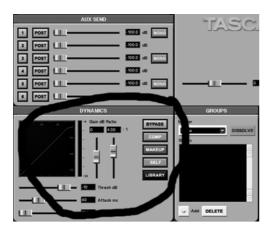
In the dynamics section, there is a button marked SELF. This is the parameter that determines which channel s signal will trigger the dynamics threshold (some compressors refer to this as the key input, key trigger or sidechain input). The default setting is SELF, which means that the dynamics processor listens to its original channel for key input (meaning that the compressor on channel 7 would look for the signal from channel 7 to trigger its input).
