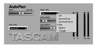
You can choose different wave shapes for modulation: Sine, Square, Triangle, Sawtooth Up, and Sawtooth Down. Try experimenting with different settings on a sound source you re familiar with —if you find one that you like, save it as a library entry.
