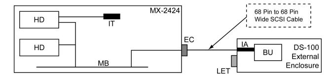
MX-2424 with standard internal hard drive, second hard drive in the front bay and a single-ended backup device (DVD-RAM or Travan) in an external 68-pin case.
