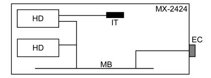
MX-2424 with standard internal hard drive and second hard drive in the front bay.
