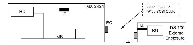
MX-2424 with standard internal hard drive and single ended backup device (DVD-RAM or Travan) in external 68-pin case.
