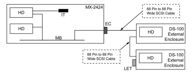
MX-2424 with standard internal hard drive, second hard drive installed in the front bay and two hard drives connected in external 68-pin cases.
