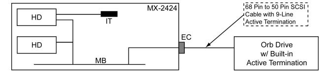
MX-2424 with standard internal hard drive, second hard drive in the front bay and an external Orb drive.
