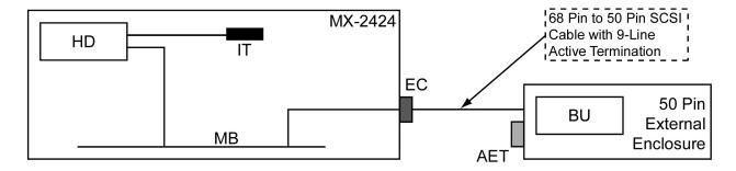
MX-2424 with standard internal hard drive and single ended backup device (DVD-RAM or Travan) in external 50-pin case.
