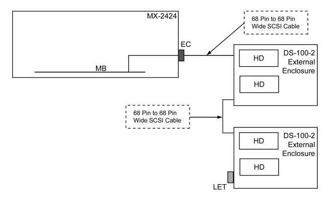
MX-2424 with internal hard drive removed/disconnected and four hard drives connected externally in 68-pin cases.
