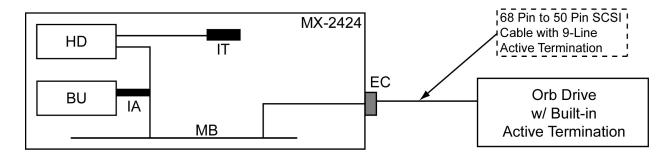
MX-2424 with standard internal hard drive, single ended backup device (DVD-RAM or Travan) in the front bay and external Orb Drive.
