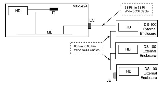
MX-2424 with standard internal hard drive and three hard drives connected in external 68-pin cases.
