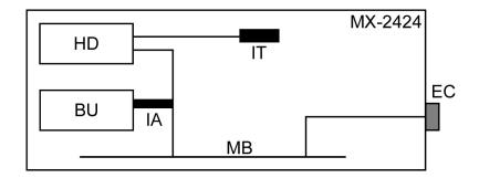
MX-2424 with standard internal hard drive and single ended backup device (DVD-RAM or Travan) in the front bay.
