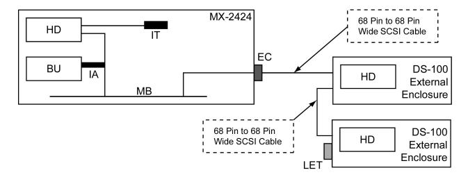
MX-2424 with standard internal hard drive, single ended backup device (DVD-RAM or Travan) in the front bay and two external hard drives.
