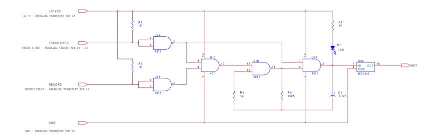
U1 - CD4011 U2 - CD4011 U3 - MC1413 OR ULN2003 ALL RESISTORS +-5%, 1/4 WATT
