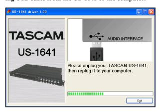
9 When the screen below appears, reconnect the US-1641 to the computer with the USB cable.
