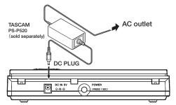
When using the AC adapter, "**\***" appears in the upper right of the display.
