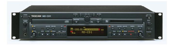
The TASCAM MD-CD1 is a 2U rack-mountable single CD player, with a powered loading tray, and MiniDisc player/recorder. The combined features provide continuous playback between MiniDisc and CD player. Disc can be duplicated from CD to MiniDisc. Remote control (RC-MC1) is included and RS-232 external control is provided (DB9 connector).
