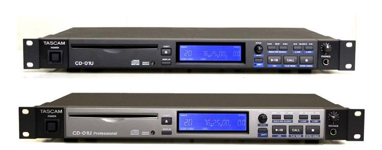
The CD-01U / CD-01UPRO are 1U rack mountable CD players with **slot loading** transports. The CD players provide multiple playback modes, auto cueing, auto-ready, Intro-Check, Pitch Control (+/- 12%), Key Original Function, and fade in/out function (up to 10 seconds in ½ step increments). The CD players are equipped with 20 seconds of RAM buffer for shock protection and both are RS-232 controllable.
