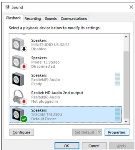
3. On the Playback tab, select "Speakers (TASCAM TM-250U)" and open the Properties window. Click on the Levels tab.
