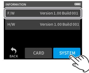
F/W shows the firmware version. Updating is not necessary if the firmware version shown here is the same or newer than the intended update version.
