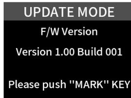
3. Press the MARK button to show the current version and build number used by the unit and the update firmware version and build number on the SD card.
