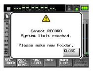
In addition, in these cases, Rec Limit appears as the remaining recording time for the currently selected CF card.
