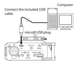
The USB SELECT screen appears when the unit is connected by USB and when the unit is turned on if the USB cable is already connected. On this screen, choose between USB bus power supply or USB connection with the computer.
