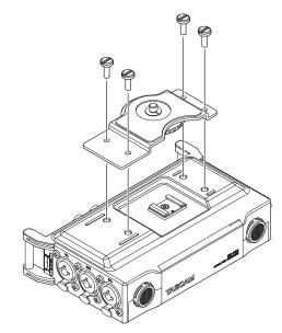
You can attach the included camera attachment bracket screw hole covers to the screw holes.
