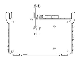
35 **Tripod mounting thread (1/4-inch)** Use to attach this unit to a tripod.
