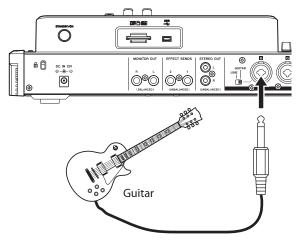
2. Set the LINE-GUITAR switch to GUITAR on the rear panel.
