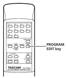
The unit enters program setting mode, and if no program has been set, it will be possible to set a track to program step 01 (MEMORY indicator blinks).
