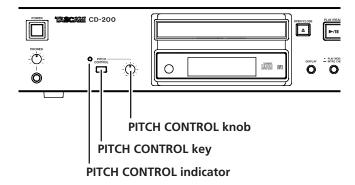
1. Press the **PITCH CONTROL** key on the main unit to turn pitch control playback ON.
