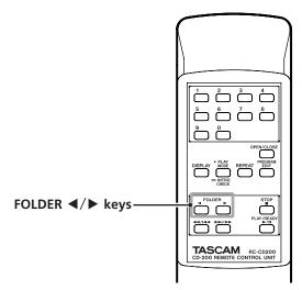
When using a data CD, by pressing the **FOLDER**  $\blacktriangleleft/\triangleright$  keys on the main unit or the remote control, you can skip to the previous or next folder. This will skip to the beginning of the first track in the previous or next folder. If you hold down one of these keys, you can skip through folders continually.
